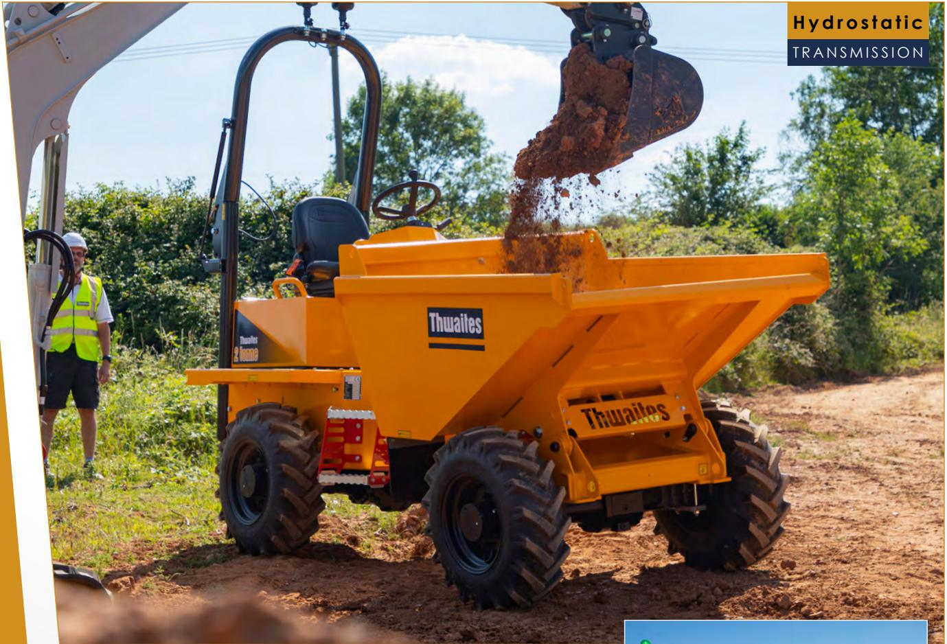
The Thwaites 2 Tonne Front Tip, Stage V dumper is manufactured with contractors and hirers in mind – ensuring operator safety, reducing risk on site and improving performance. Powered by an 18.4 kW 3-cylinder Yanmar engine, delivering 107 Nm max torque for optimum traction and control. The Thwaites 2 Tonne Front Tip is also available with a Manual Transmission.
