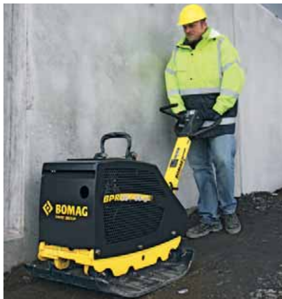
BPR 35/60 D with optional all-round protection hood: prevents site damage.
